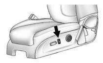
On vehicles with seats that have power reclining seatbacks, the controls used to operate them are on the outboard side of the seats.
